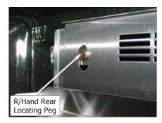
Tilt the top of the rack inwards and lift the rack off the lower mounting brackets.
